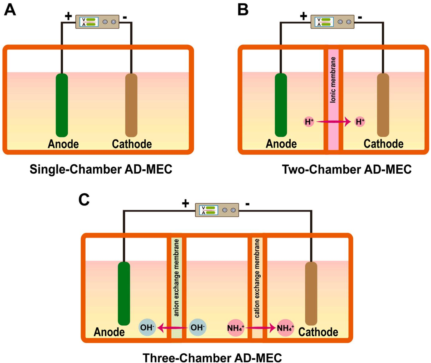
Fig. 7. Configurations of AD-MEC systems with single chamber (A), two chambers (B), and three chambers (C).
