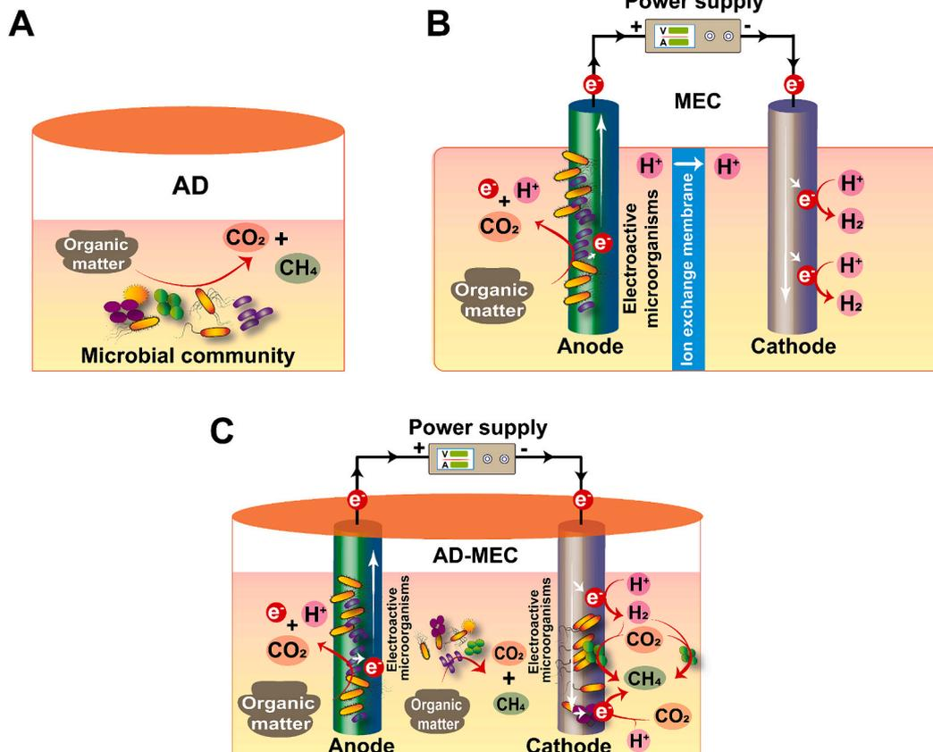
Fig. 1. Schematic diagrams for AD (A), MEC (B), and AD-MEC (C).
